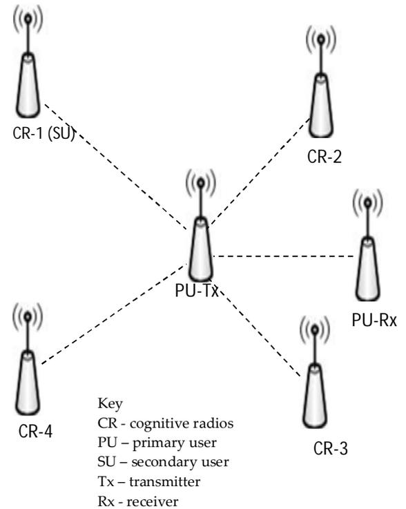
Fig. 2 Cognitive Radio Network with Multiple Radios
