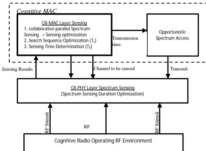
Fig. 3 CRN cross-layer optimized structure
