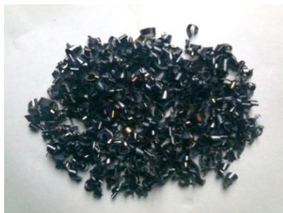
Figure 4.1. Steel Fibre from Laths Machines
