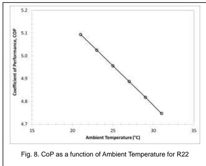
Fig. 8. CoP as a function of Ambient Temperature for R22
