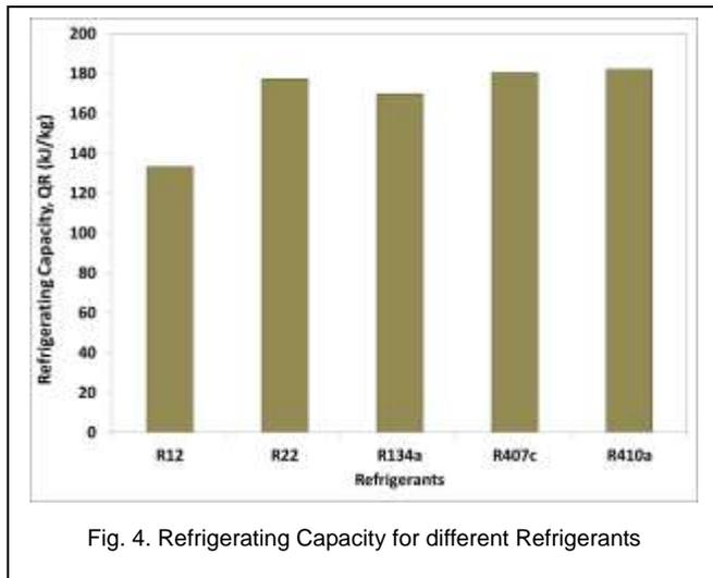
Fig. 4. Refrigerating Capacity for different Refrigerants
