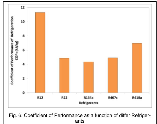
Fig. 6. Coefficient of Performance as a function of differ Refrigerants
