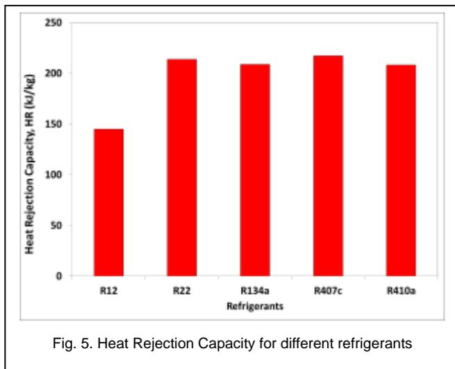
Fig. 5. Heat Rejection Capacity for different refrigerants
