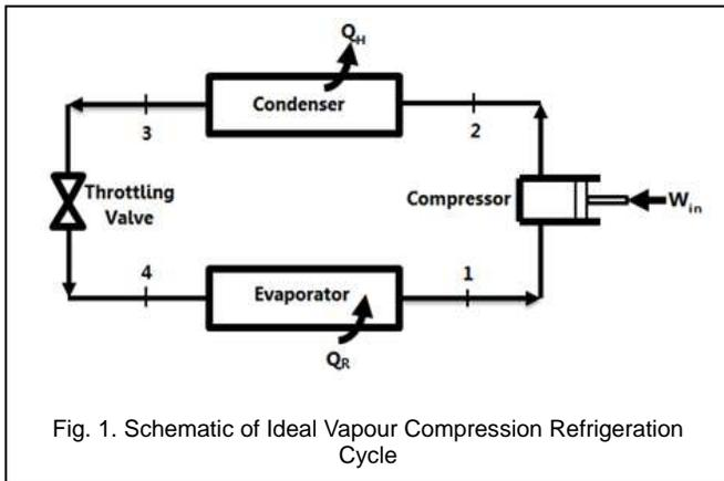
Fig. 1. Schematic of Ideal Vapour Compression Refrigeration Cycle
