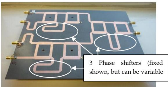
Fig.1b: PCB microstrip beam shaping network @uplink frequency band
