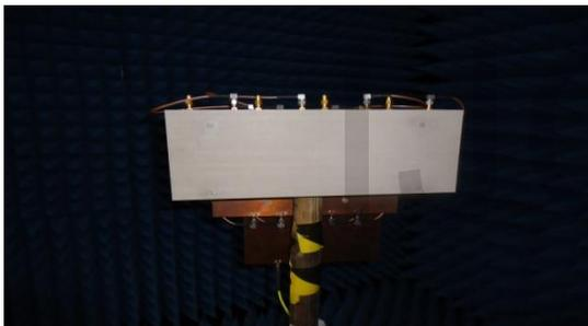
Fig.1a: Multiple switched beams smart with beam shaping and WAIM sheet covering top of the array antenna capability in ane-
