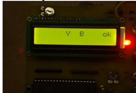
R faulty and Y B ok
