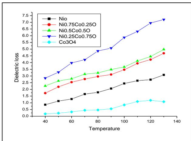
Fig.6. Dielectric Loss for various Temperature and constant frequency 1Kz for all Composites
