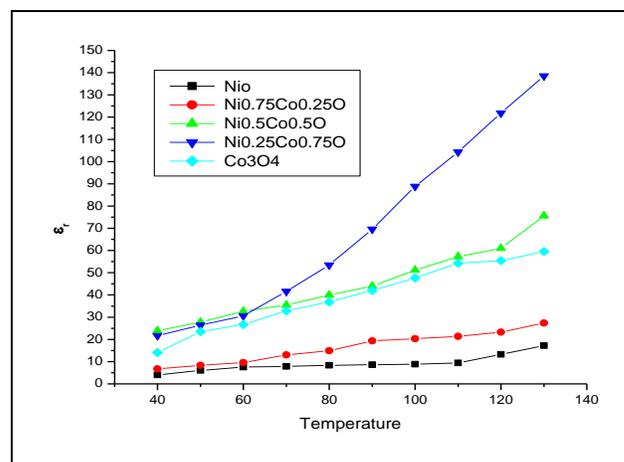
Fig. 5. Dielectric constant for various Temperature and constant frequency 1Kz for all Composites
