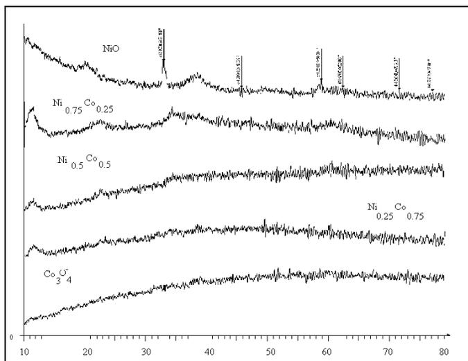
Fig. 1. XRD image for the Ni<sub>x</sub>Co<sub>(1-x)</sub>O composites
