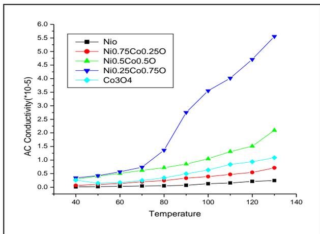
Fig. 7. AC conductivity for various Temperature and constant frequency 1Kz for all Composites
