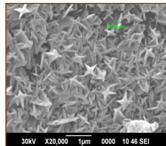
Fig. 4. The SEM image for Ni<sub>x</sub>Co<sub>(1-x)</sub>O compounds
