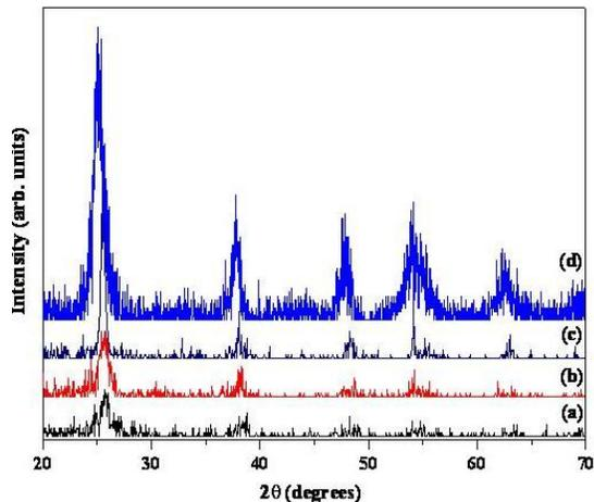
**Figure 1: XRD pattern of TiO<sub>2</sub> nanoparticles prepared by sol gel method (a) as prepared (b) calcined at 300 °C (c) 600 °C (d) hydrothermally prepared and annealed at 600 °C.**
