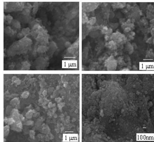
**Figure 2: SEM image of TiO<sub>2</sub> nanoparticles prepared by sol gel method (a) as prepared (b) calcined at 300 °C (c) 600 °C (d) hydrothermally prepared and annealed at 600 °C.**
