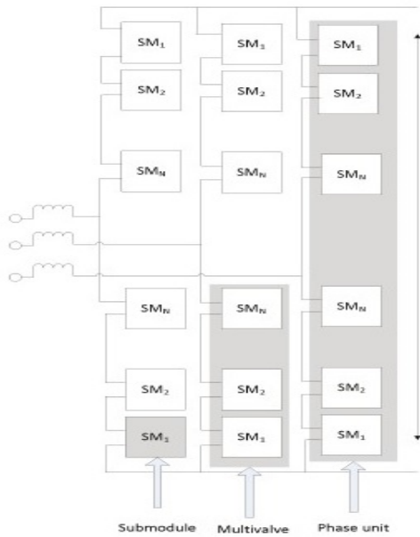
Figure 2.2 (a) The MMC Structure
