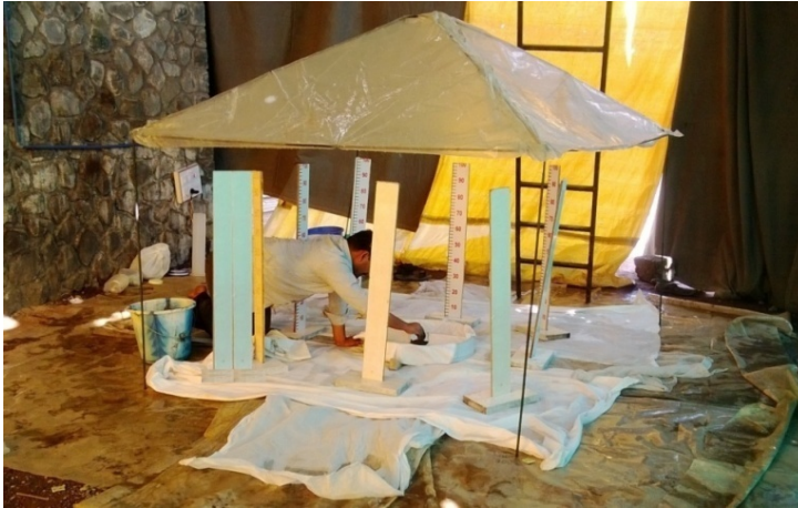
Fig.1 Complete arrangement for quantification of splashed soil.
