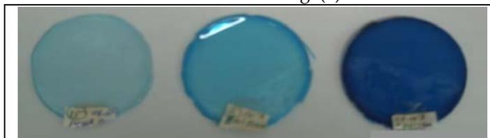
The thickness of the films produced by this method is dependent on concentration and the volume of the liquid in the dish. The liquid volume was (10) ml, yielding film of different thickness.
