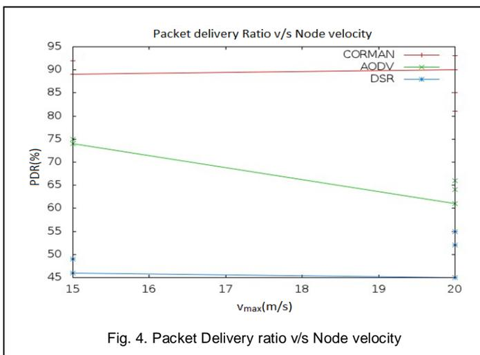
Fig. 4. Packet Delivery ratio v/s Node velocity
