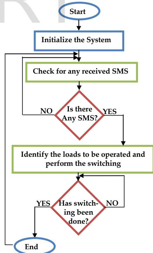
Fig.5. Flowchart of the switching
