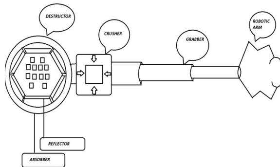
Fig. Space debris destructor equipment
