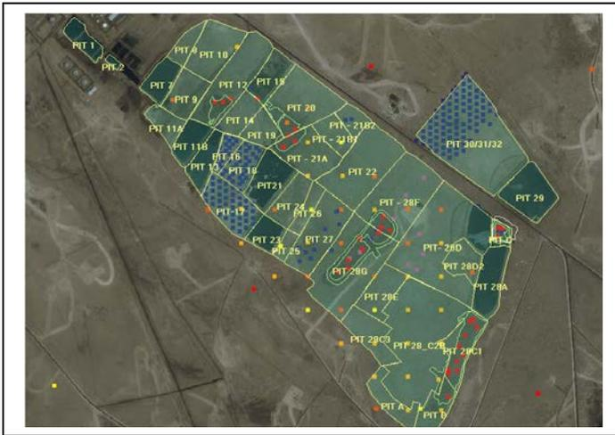
Fig. 1. Wafra Main Gathering Center area indicating evaporation pond boundaries and stockpile locations.
