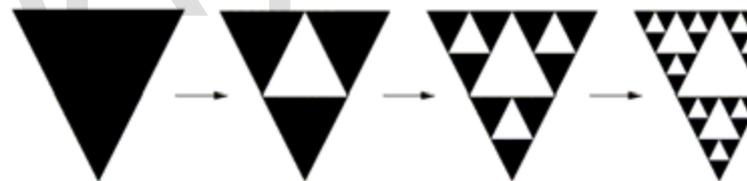
Fig. 1- Generation of Sierpinski Antenna Pattern
