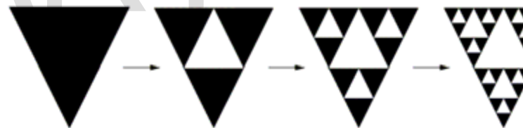
Fig. 1- Generation of Sierpinski Antenna Pattern
