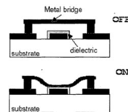
Fig. 5- Side view of a shunt MEMS switch
