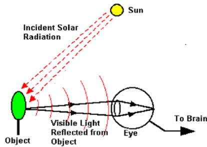
Figure 2: Visual Remote Sensing System
