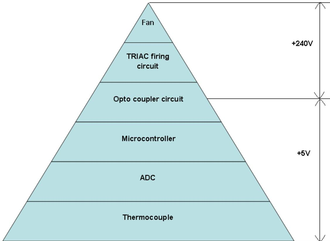
Simple circuit structure diagram
