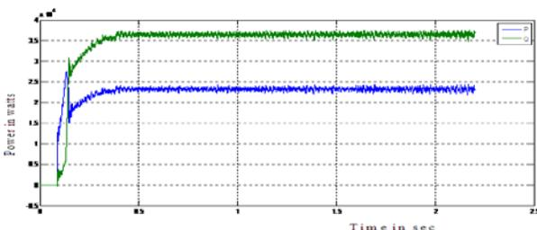
Figure 5.2.6 shows the reversal of active power (P) and reactive power (Q) flows in the power system after integration in the power system
