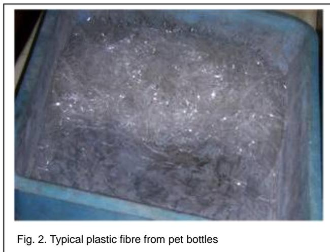
Fig. 2. Typical plastic fibre from pet bottles
