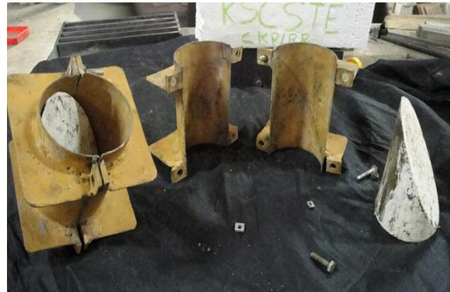
Figure 2. Mould of specimens used for slant shear test
