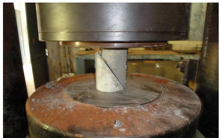
Figure 3. Specimen subjected to slant shear test
