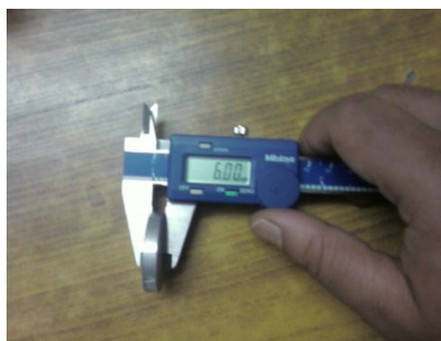
Fig.1 (c) Prepared workpiece of Al/SiC-MMCs
