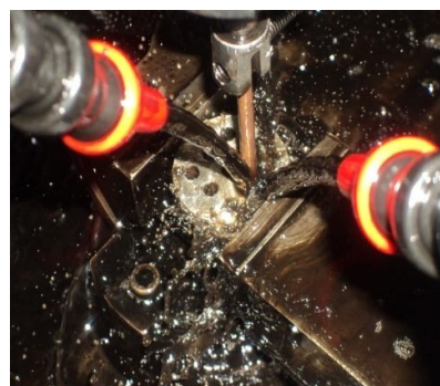
Fig.2(b) Machined number of holes by EDM
