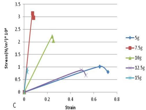
Fig. 3. Stress-Strain curves for (A) pure polyethylene (B) blended Polyethylene (c) waste polyethylene
