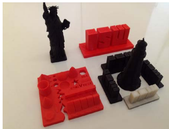
Figure 1: Examples of plastic components produced by the 3D printer designed and manufactured at ISW
