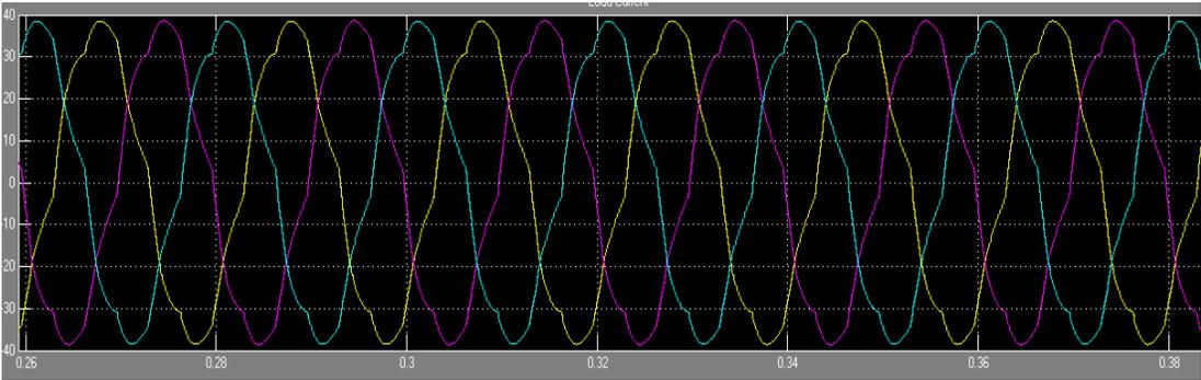
Figure 7 Load voltage and current waveform (a,b,c)
