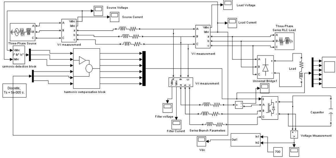
Figure.5 Simulation Model of Hysteresis Current Control
