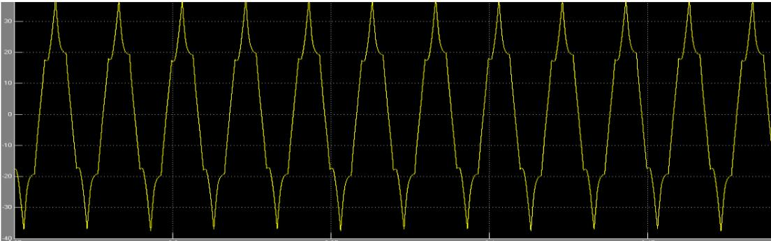
Figure 8 Distorted Line Current
