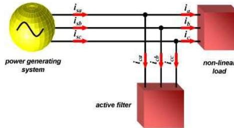
Figure.1 Shunt Active Power Filter
