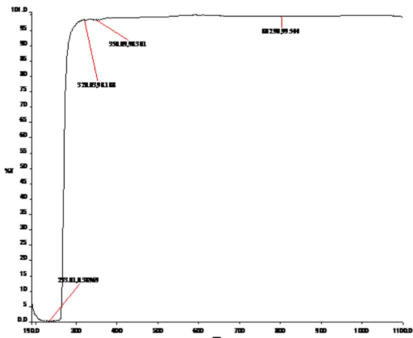
Fig.4. UV Transmission Spectrum of ZTS doped with KI
