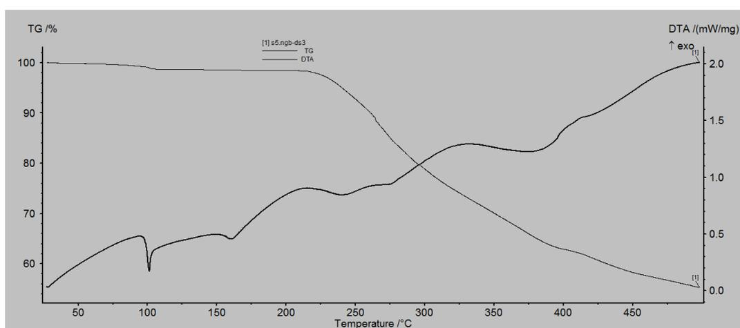
Fig.5. TGA/DTA of ZTS doped with NaCl
