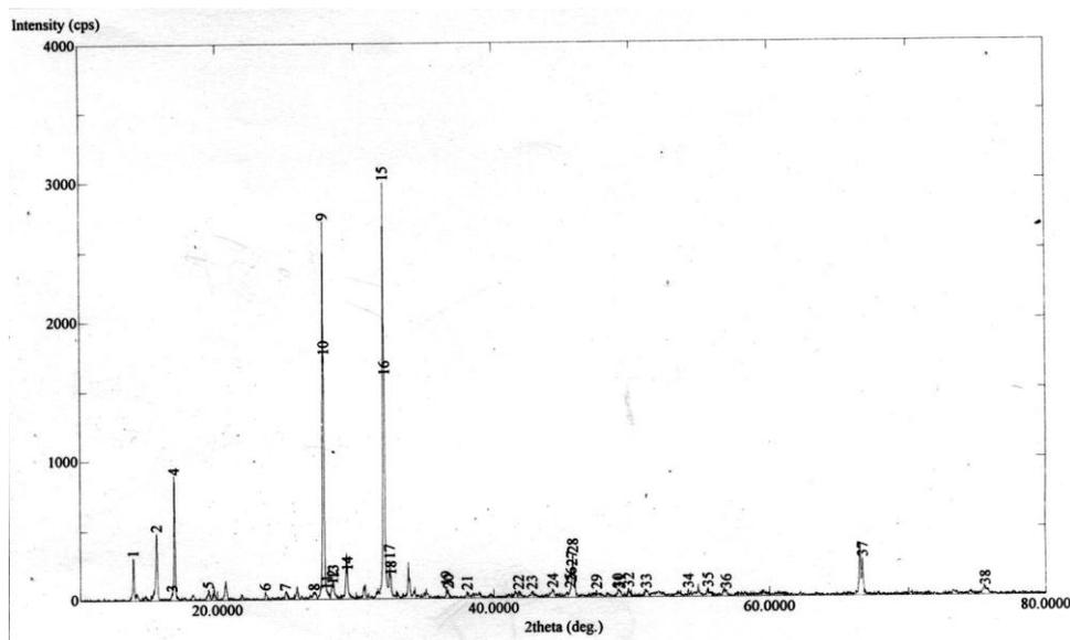
Fig.1. XRD Pattern of ZTS doped with NaCl
