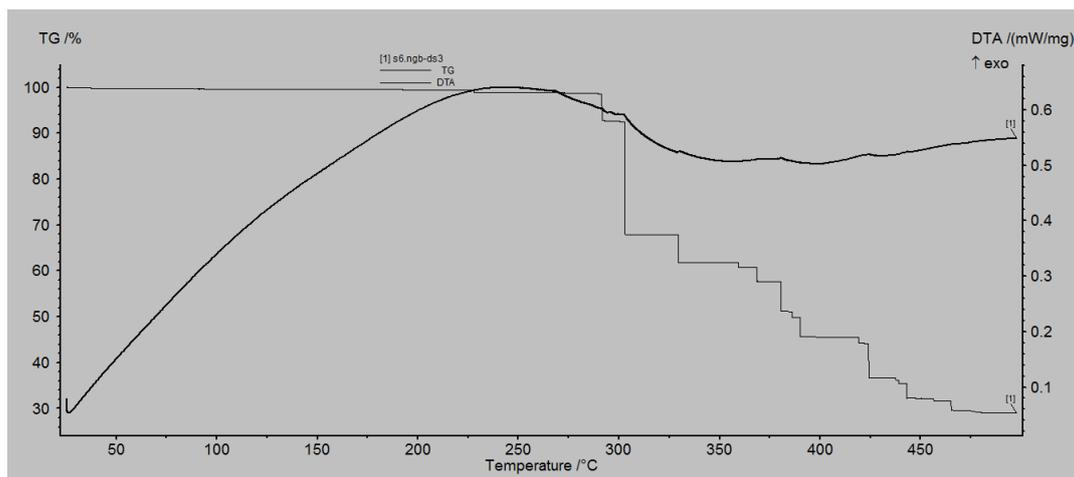
Fig.6. TGA/DTA of ZTS doped with KI
