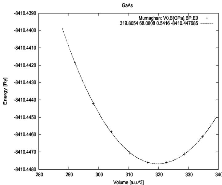
Fig 4: Volume optimization plot of GaAs.
