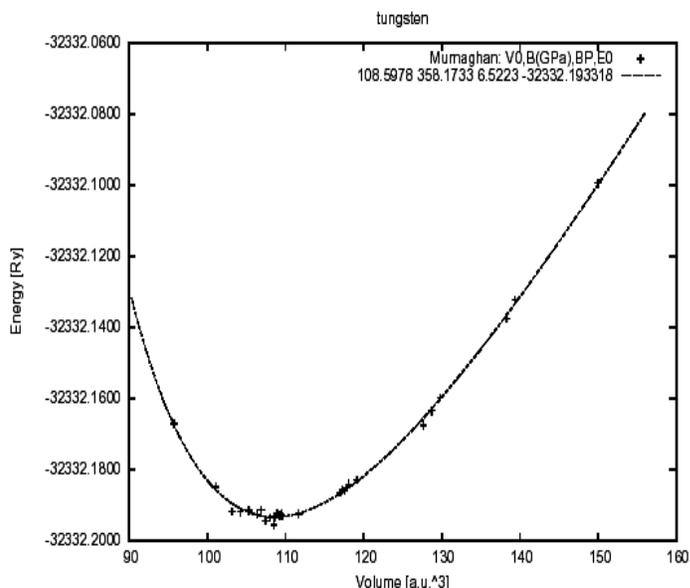
Fig 1: Volume optimization plot of W obtained by GGA calculations.
