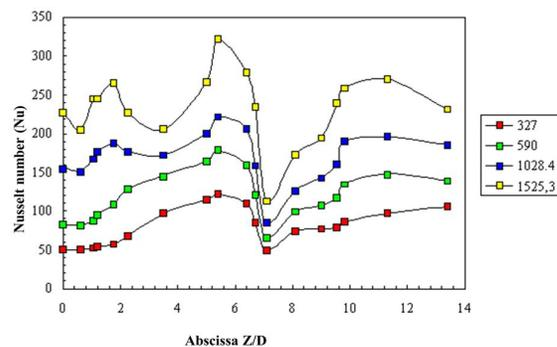
**Fig. 10 :** Evolution of Nusselt number as a function of constant volume fraction  $\phi = 10\%$  and a constant flux density  $\Phi = 9480 \text{ W/m}^2$ .
