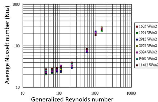
**Fig. 5 : Evolution of the average Nusselt number function of different values of heat flux densities.**
