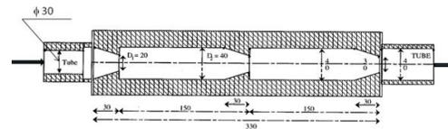
**Fig.2: Complex geometry of the test section.**
