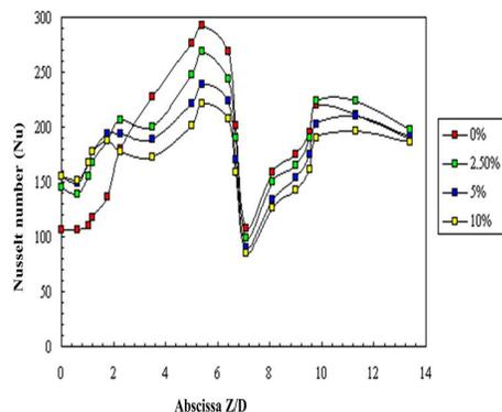
Fig. 12: Evolution of Nusselt number as a function of constant Reynolds number  $Reg = 1028$  and a constant flux density  $\phi = 9480 \text{ W/m}^2$
