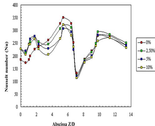
Fig. 13: Evolution of Nusselt number as a function of constant Reynolds number  $Reg = 1525$  and a constant flux density  $\phi = 9480 \text{ W/m}^2$
