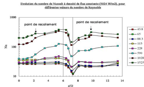
Fig.6 : Evolution of the Nusselt number at constant heat density flux equal 5024 W/m2 for different values of the generalized Reynolds number Reg.
