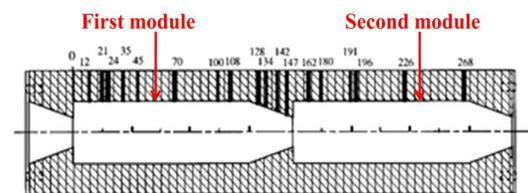
**Fig.3b: Location and grading of thermocouples**
