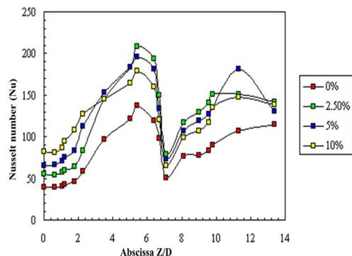
Fig. 11: Evolution of Nusselt number as a function of constant Reynolds number  $Reg = 590$  and a constant flux density  $\phi = 9480 \text{ W/m}^2$
