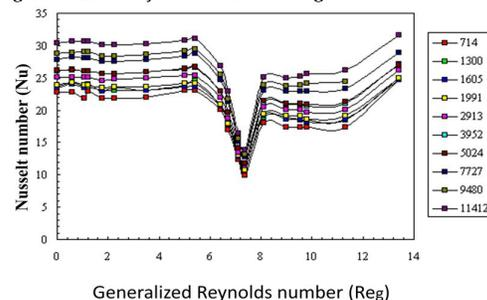
Fig. 7 : Evolution of the Nusselt number as a function of different heat flux for a constant generalized Reynolds number ( $Re_g$ ) equal to 43.8
