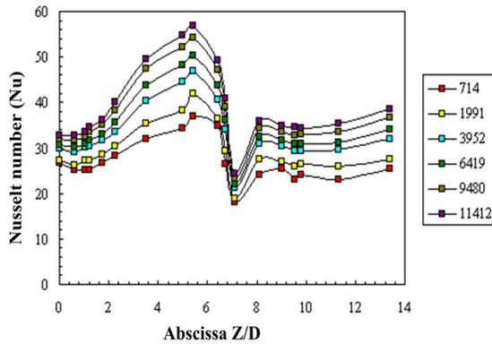
**Fig. 8 :** Evolution of the Nusselt number as a function different heat flux for a constant generalized Reynolds number (Reg) equal to 228.
