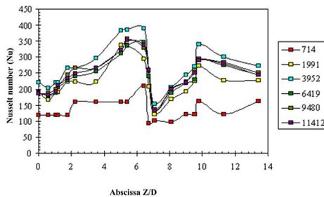
**Fig. 9 :** Evolution of the Nusselt number as a function different heat flux for a constant generalized Reynolds number (Reg) equal to 1525
