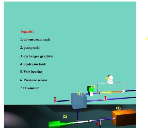
**Fig.1: Schematic of test loop**
