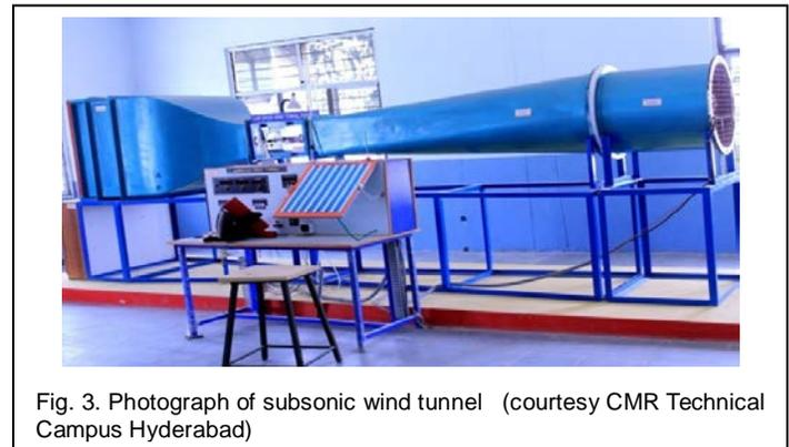
Fig. 3. Photograph of subsonic wind tunnel (courtesy CMR Technical Campus Hyderabad)
