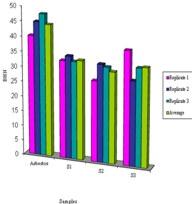
2. Figure 2. Comparison of BHN of asbestos and PKS based friction composites: S<sub>1</sub>, S<sub>2</sub>, S<sub>3</sub> are PKS based samples
