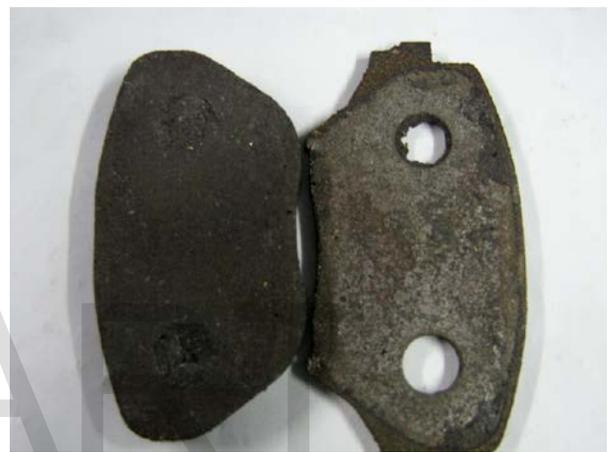
b) PKS-base Friction Composite Brake Pad Sample
