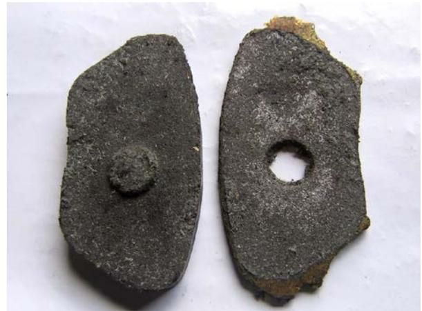
a) Asbestos-base Friction Composite Brake Pad Sample
