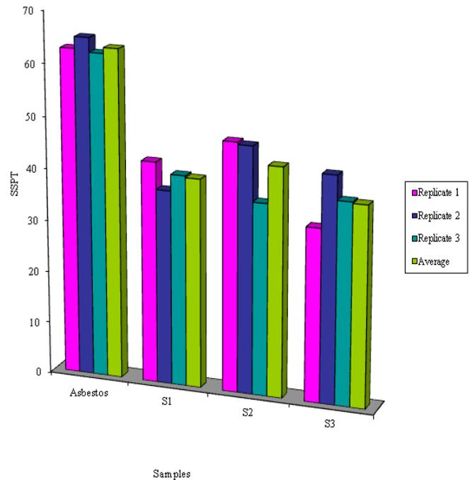
Figure 3. Comparison of SSPT of asbestos and PKS base friction composite: S<sub>1</sub>, S<sub>2</sub>, S<sub>3</sub> are PKS based samples
