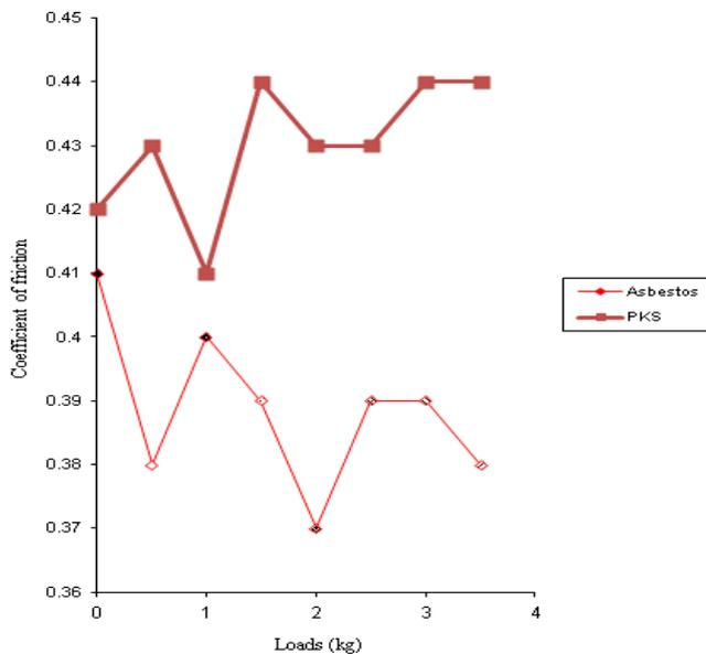
Figure 4. Comparison of coefficient of friction of asbestos and PKS based friction composite
