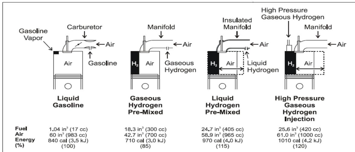
Fig 3 (C) : Mixing Proportion of Hydrogen with Gasoline
