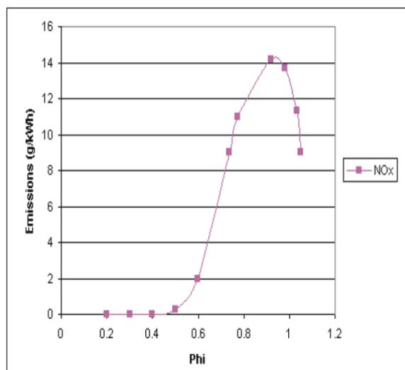
Fig 4(II) - Emissions of Hydrogen Engine
