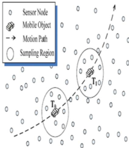
Fig. 1. Sensor field sampling.
