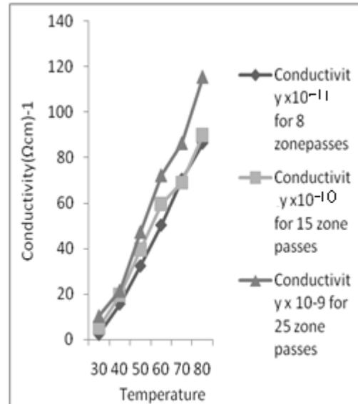
Fig. 3: Temperature v/s Conductivity with Zone passes for CdI<sub>2</sub> crystal
