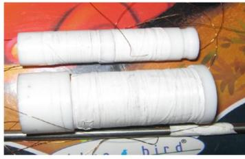
Fig 1. Picture of the ac susceptometer (Above one is the primary coil and below one is the secondary coil wrapped with the Teflon tape)
