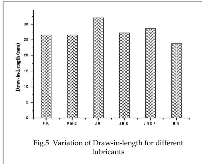
Fig.5 Variation of Draw-in-length for different lubricants
