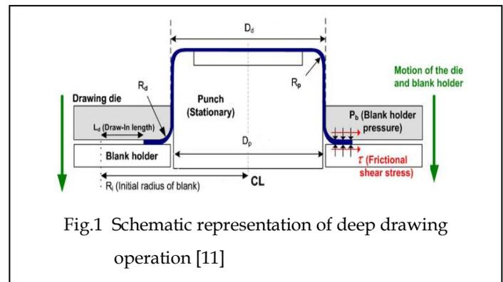
Fig.1 Schematic representation of deep drawing operation [11]
