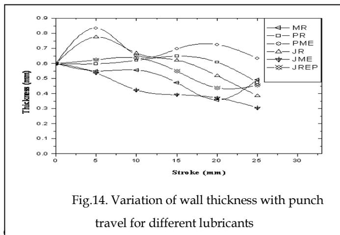
Fig.14. Variation of wall thickness with punch travel for different lubricants
