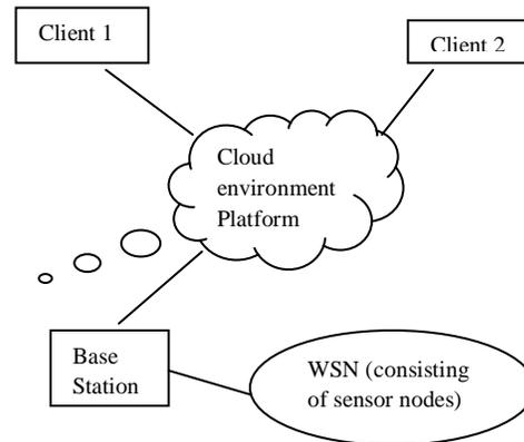
Fig 1: Block diagram of WSN in cloud environment
