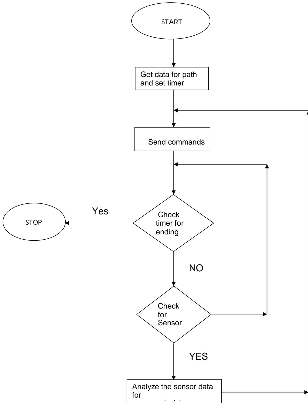
FIG. 2 - Flowchart for the vehicle control
