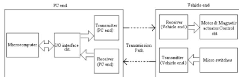
Figure 1 - simple block diagram of the complete system
