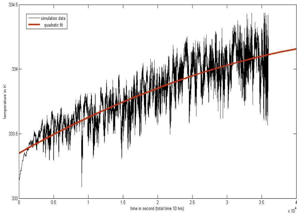
Fig. 11: Plot of temperature rise by 1°C while heater is on inside the storage tank at the centre of the tank.
