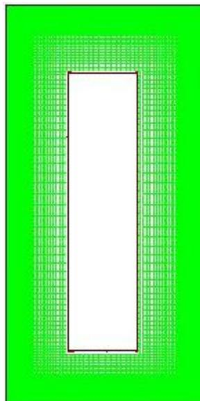
Fig.6: Complete 2-D view of geometry with central heater with mesh size 18,360.
