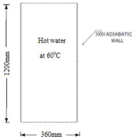
Fig.2: Schematic diagram of the Hot Water Storage Tank under study.
