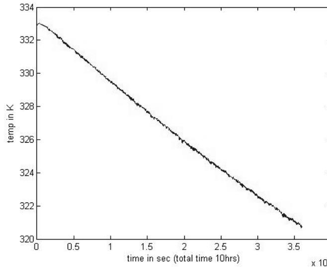
Fig.8: Time v/s temperature plot in the tank when heater is OFF and temperature drop from the tank.
