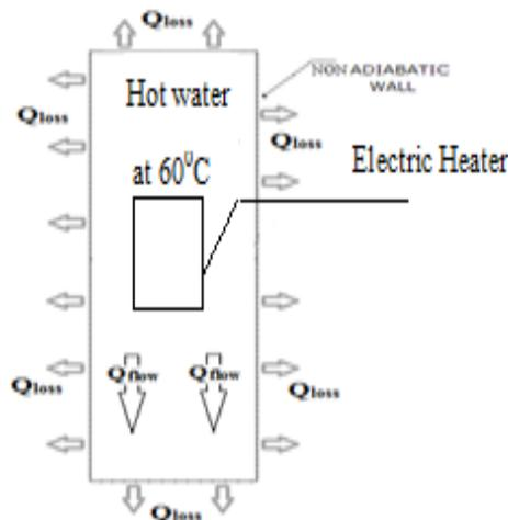
Fig. 4: Hot water tank at constant temperature with electric heater.
