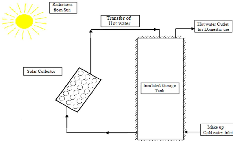
Fig.1: Schematic diagram of SDHW system.
