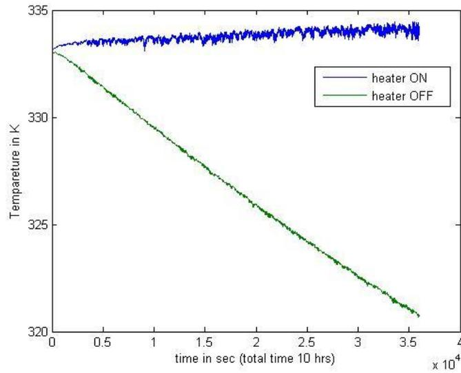
Fig. 10: Plot of comparison when heater is ON and OFF in the storage tank
