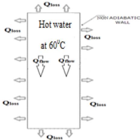
Fig. 3: Hot water in the tank at constant temperature.
