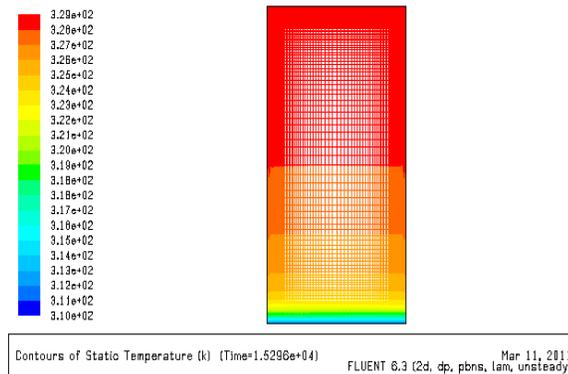
Fig. a: Temperature contour after 04 hours.
