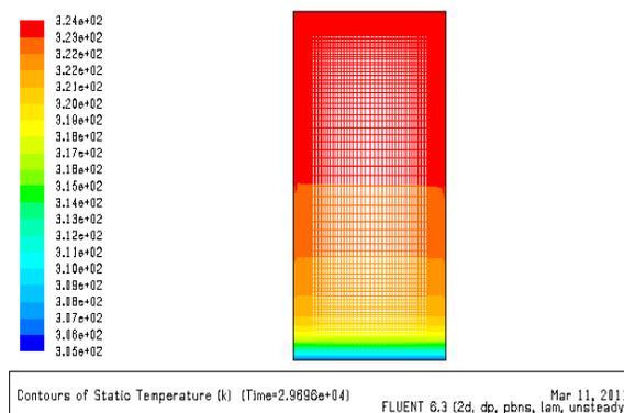
Fig. a: Temperature contour after 08 hours.
