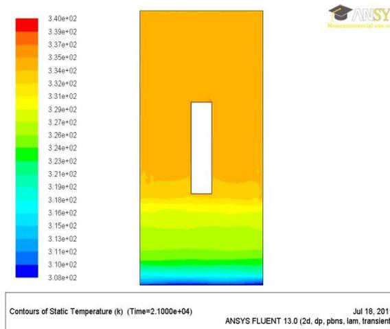
Fig. b: Temperature contour after of 06 hours.
