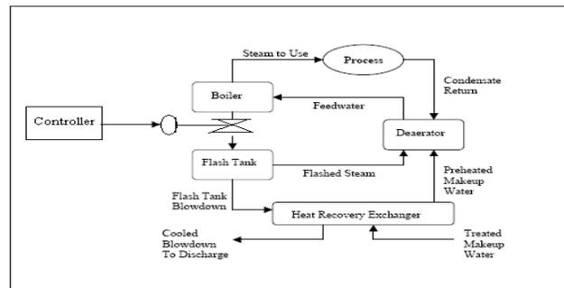
Fig. 2 Conventional method of control
