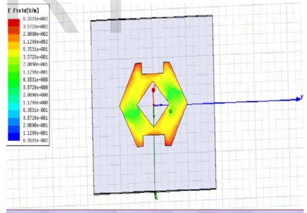
Fig2:-Main design with hexagonal patch
