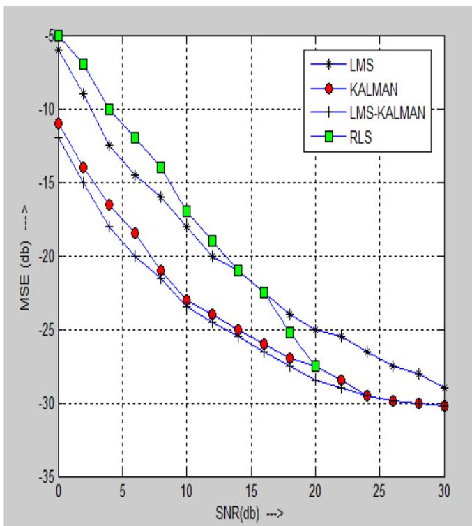
Fig.6 Simulation Result of SNR Vs MSE for various adaptive algorithms
