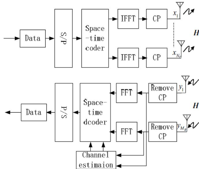
Fig.1 MIMO-OFDM System for adaptive channel estimation in [2]
