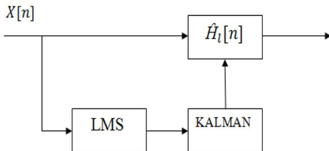
Fig. 5 Adaptive channel estimation based on LMS +KALMAN [5]
