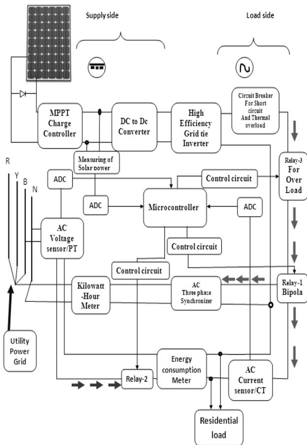
Fig. 5 Grid-Tied PV system block diagram.
