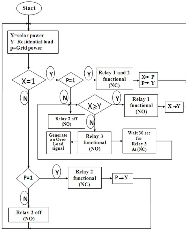
Fig. 7, Flow chart of the control scheme
