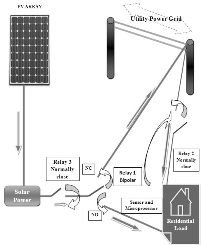
Fig. 4 Schematic diagram of the planed grid-tied PV system
