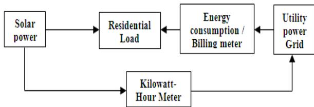
Fig. 8, Net metering system
