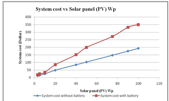
Fig. 9. System cost vs. solar panel (PV) Wp
