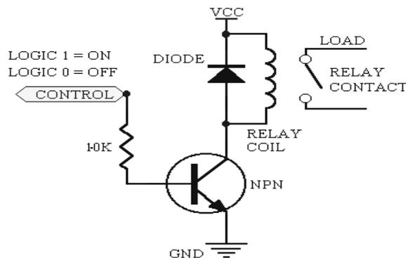
Fig. 6 Relay control circuit.
