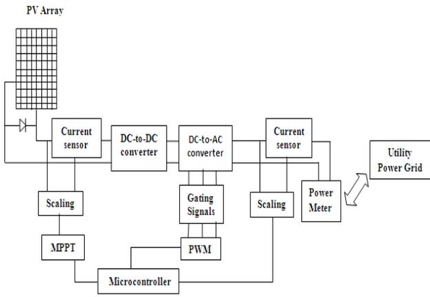
Fig. 2 Block diagram of a grid-tied PV system
